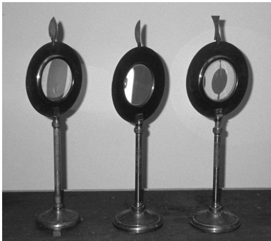
Lens Set. These three lenses are in regular use in lecture demonstrations at the University of Cincinnati physics department. The sheet brass outlines show that the lenses are double-convex (converging), plano-convex (converging) and double-concave (diverging). The set is marked Jules Duboscq/Ph PELLIN/Paris. Jules Duboscq (1817–1886) was succeeded in business by Phillippe Pellin. (Photograph and Notes by Thomas B. Greenslade, Jr., Kenyon College)
